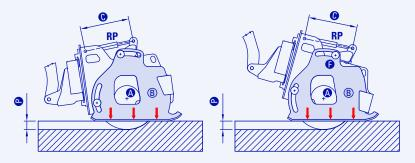
The depth adjuster **RP** (mechanical or hydraulic) moves the fulcrum 1 up and down, determining the working depth 2. If the planer is not horizontal to the surface, the side 1 rotates forward or rearward comparing to the virtual axis 1; the lateral skis are this way always adherent to the surface and the working depth 2 stays constant while advancing. The working depth 2 can be modified only by changing the stroke 3 of the depth adjuster **RP**.
